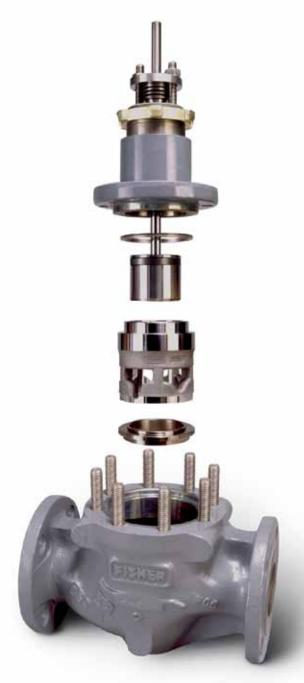
**Quick-Change Trim Means Fast Service** The easy-e control valve's quick-change, cage-style trim reduces the maintenance challenge, which increases operating time and reduces operating expense.
