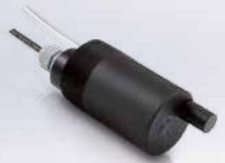
OPTISENS TUR 2000 90° scattered light sensor for turbidity measurements with NIR-LED for long-term stability and automatic cleaning
